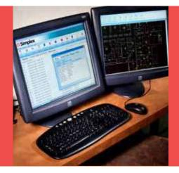
The TrueSite system is further distinguished by its exceptional survivability. Unlike some other systems, the TrueSite workstation operates as an actual node on the network. This architecture has an advantage of providing true peer-to-peer linkage with all panels on the network, thereby fortifying the TrueSite system's ability to continue operations even if a catastrophic event cripples other parts of the network.
