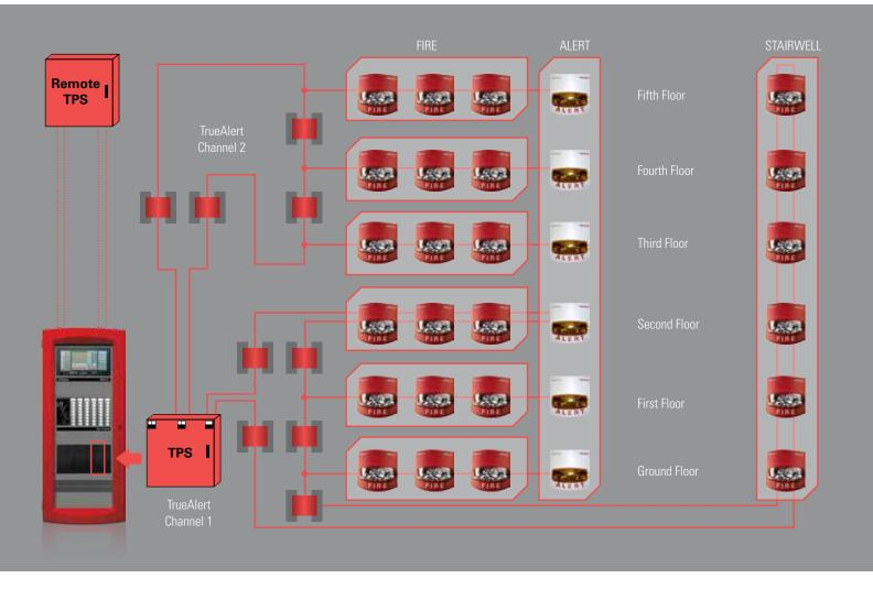
When controlled from a Simplex 4100ES control panels with TPS, additional features are available such as software selection strobe intensity, detailed reports of actual appliance intensity selection, TrueNAC voltage drop diagnostics and additional setup and test diagnostics.
