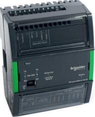
The Automation Server is a powerful device that can act as a standalone server and also control I/O modules and monitor and manage field bus devices.
