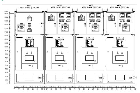
MV panel comprises of One protection PIX panel and 3 metering PIX panel.
